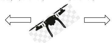
**Adjusting Roll** (Roll the Drone Left/Right)
